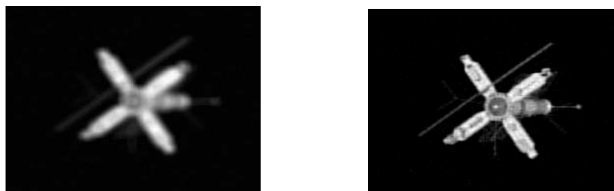
Figure 3: Satellite image with motion blur. The PSNR increases from 142.688 in the received image to 147.510 in the restored image.
